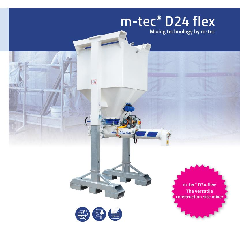
The m-tec® D24 flex is a versatile m-tec continuous mixer with maximum adaptability for a wide range of materials and feed rates. It combines the best features of the proven m-tec® D20 SN and D40 models – hence the name "D24 flex".
